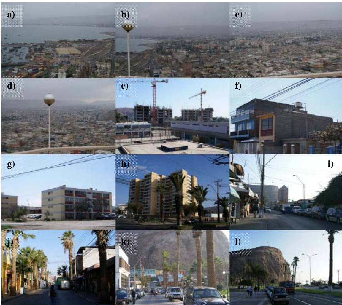
Figure 3. Pictures from visits to Arica: a) west side, b) downtown, c) mid-east, d) east side, e) new reinforced concrete shear wall buildings near the shoreline, f) typical residential 2-storey brick masonry shear wall buildings, g) typical residential 4-storey confined masonry shear wall building, h) new typology of residential reinforced concrete shear wall building near the shoreline, i) downtown district at less than 500 meters from the shoreline, j) north view of typical commercial streets in downtown Arica, k) south view of closest structures to shoreline, and l) streets at the shore line with the view of the characteristic 130-m tall hill El Morro.
